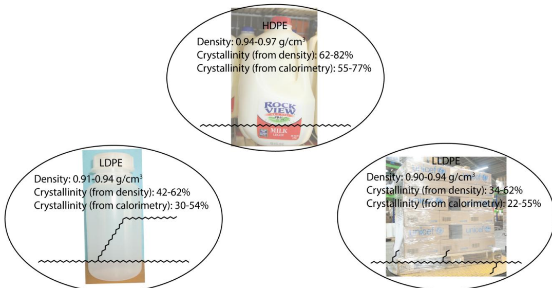
Figure 2.2. Differences in properties and applications between three major forms of polyethylene 4
